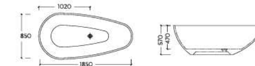
Size A 1500 X 750 X 540 mm Size B 1650 X 800 X 540 mm Size C 1700 X 850 X 530 mm Size D 1800 X 850 X 570 mm
